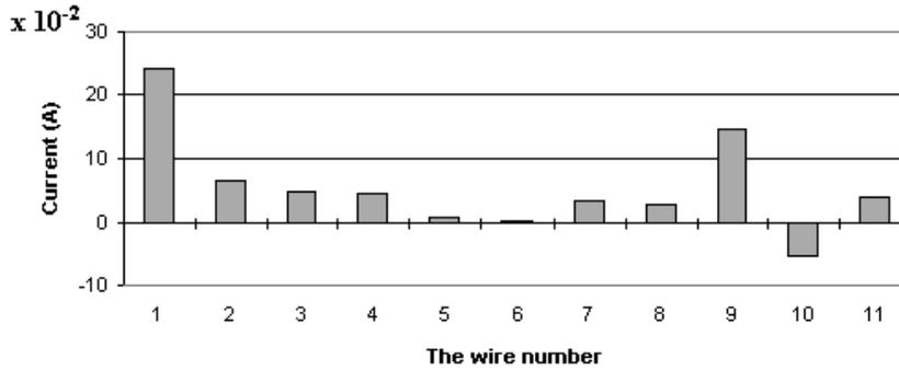
Fig. 14. Current distribution in wires of the first part of the elbow (section S2).
