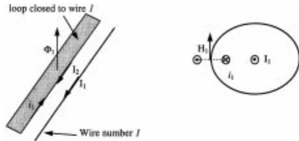
Fig. 16. Inductive crosstalk between wires.
