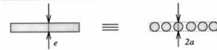
Fig. 2. The wire diameter is equal to the thickness  $e$  ( $2a = e$ ).
