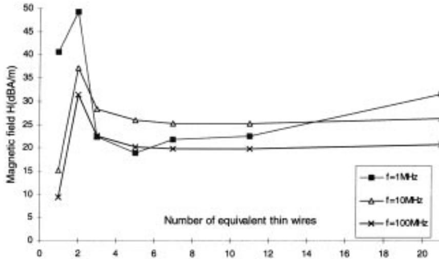
Fig. 10. Influence of wires' number on the radiated magnetic field,  $h = 15$  mm.
