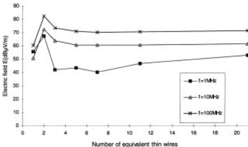
**Fig. 9.** Influence of wires' number on the radiated electric field,  $h = 15$  mm.
