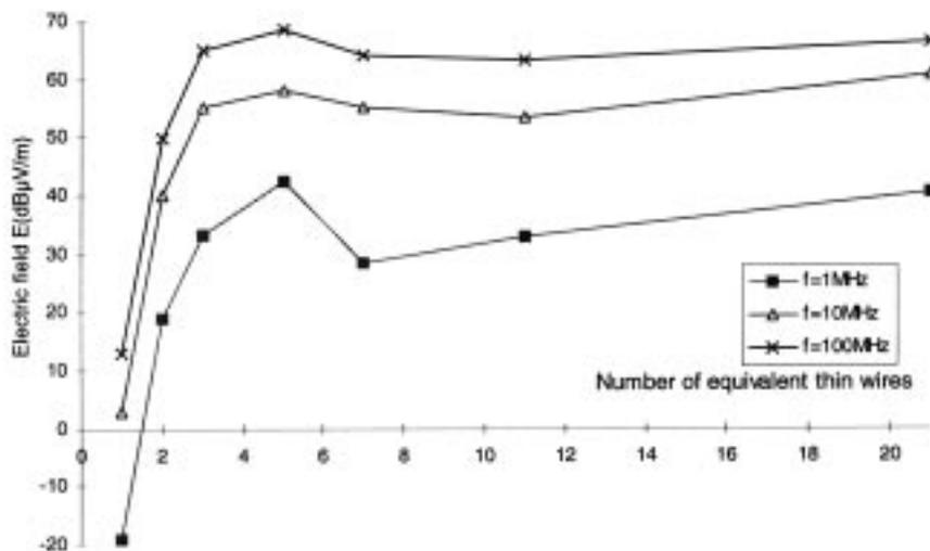
**Fig. 8.** Influence of wires' number on the radiated electric field,  $h = 1.5$  mm.
