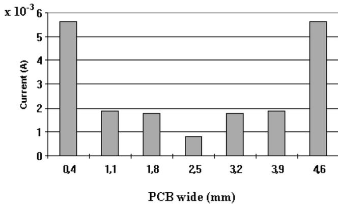
Fig. 11. Current distribution inside thin wires  $f = 100$  MHz,  $h = 15$  mm.
