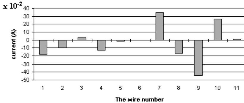
Fig. 15. Current distribution in wires of the second part of the elbow (section S3).
