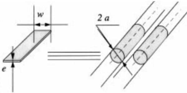
Fig. 3. The wire diameter is calculated using the PCB dimensions and  $N$ .
