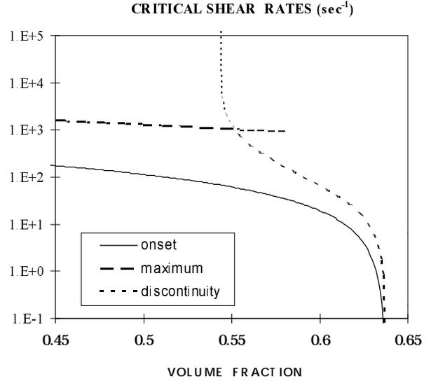
**Fig. 2.** Critical shear rates  $\dot{\gamma}_C$ ,  $\dot{\gamma}_D$  and  $\dot{\gamma}_M$  vs. volume fraction  $\phi$ , for  $\sigma_c = 1 \text{ Pa}$  (corresponding value:  $w_c \approx 3KT$ , for particle radius  $a = 0.1 \mu\text{m}$ ) (same values of model variables as in Fig. 1).
