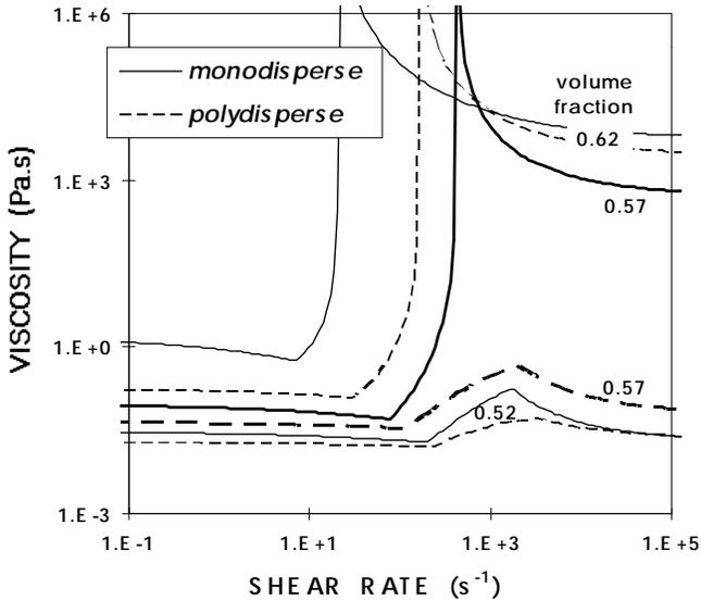
**Fig. 4.** Effect of polydispersity on model rheograms,  $\eta$  vs.  $\dot{\gamma}$  for two compactness values: monodisperse particles ( $\varphi_a; \varphi_b$ ) = (0.637; 0.525), polydisperse particles ( $\varphi_a; \varphi_b$ ) = (0.67; 0.58) (remaining model variables : same values as in Fig. 3).
