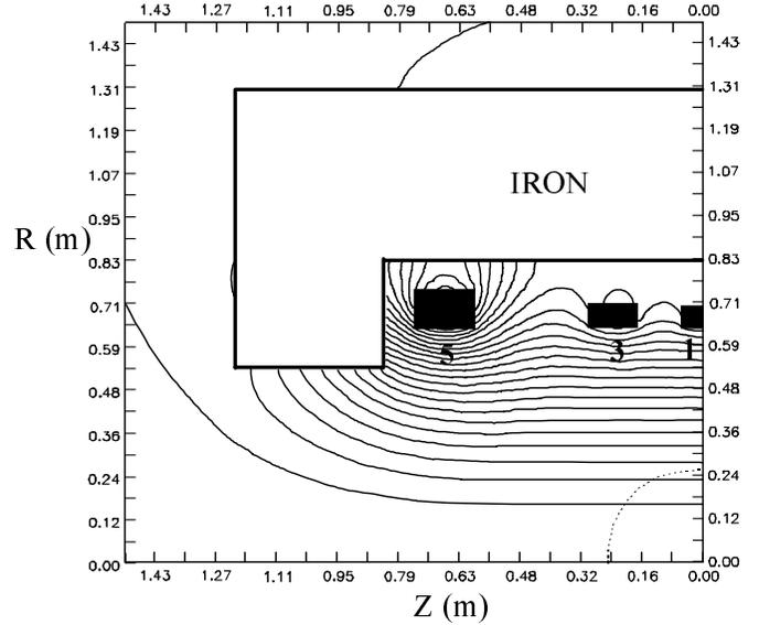
**Fig. 7.** Coil positions and dimensions and magnetic flux line distribution for the iron shielded configuration.**Table 2.** Main results for the iron shielded device.
