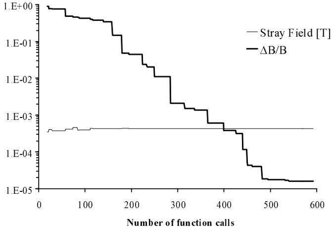
**Fig. 6.** Behavior of the field non-uniformity  $\Delta B/B$  and of the stray field  $B_s$  during the last minimization process for the iron shielded configuration.
