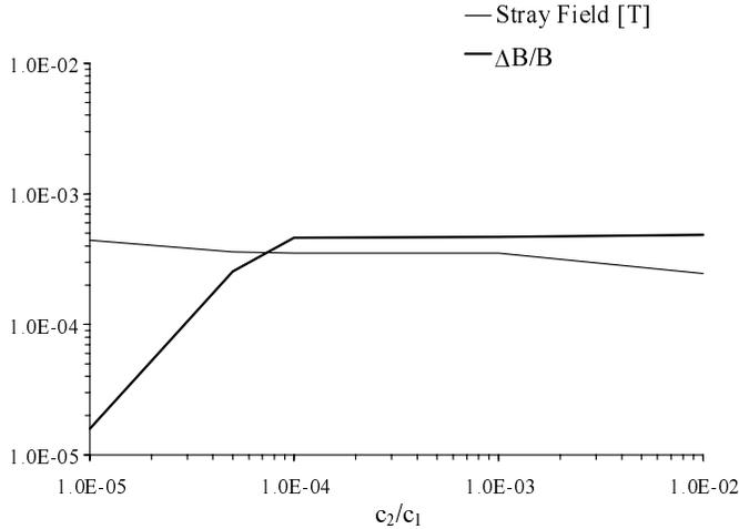
**Fig. 5.** Values at the minima of the field non-uniformity and of the stray field as functions of the penalty constant ratio  $c_1/c_2$ .
