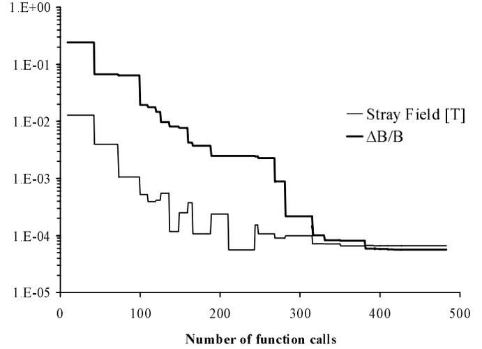
**Fig. 3.** Behavior of the field non-uniformity  $\Delta B/B$  and of the stray field  $B_s$  during the last minimization process for the actively shielded configuration.
