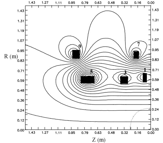
**Fig. 4.** Coil positions and dimensions and magnetic flux line distribution for the actively shielded configuration.
