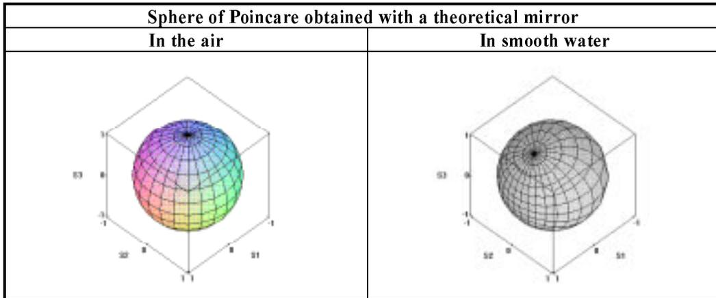
Poincare representation is a sphere with a unit radius. As previously indicated the diattenuation is noticeable on this representation: it is characterized by the poles which are getting closer.
