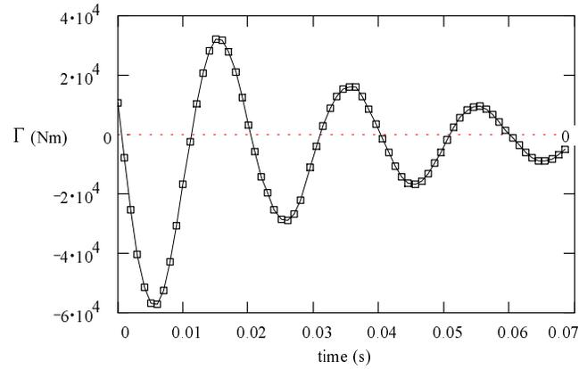
Fig. 6. Short circuit torque waveforms.
