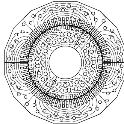
Fig. 7. Flux distribution at the initial time of the short circuit.
