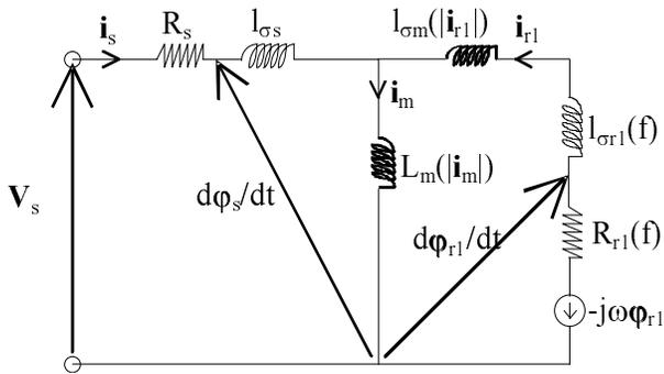
Fig. 3. Equivalent circuit of a saturated induction machine in a stator reference frame.
