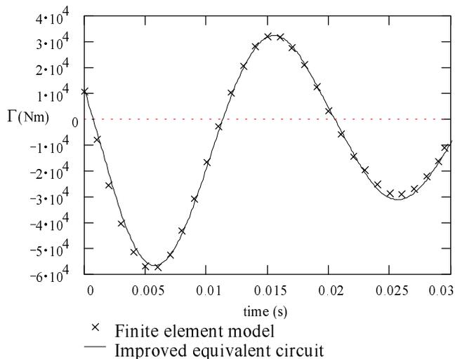
Fig. 13. Three phase short circuit torque.
