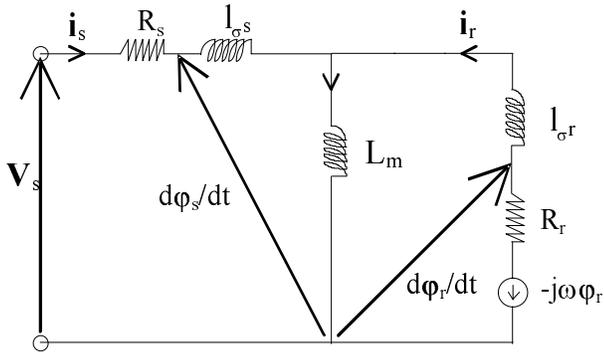
Fig. 2. Equivalent circuit of a single cage induction machine in a stator reference frame.
