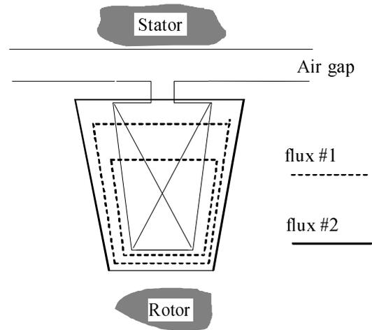
**Fig. 12.** Rotor bar leakage flux paths.
