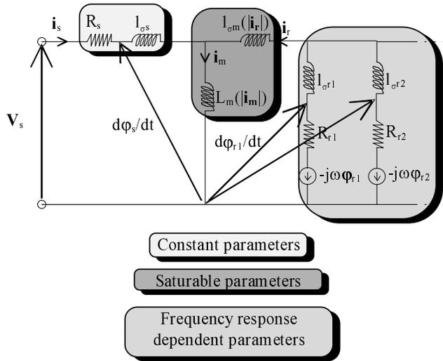
**Fig. 11.** Improved equivalent circuit of a cage induction machine.
