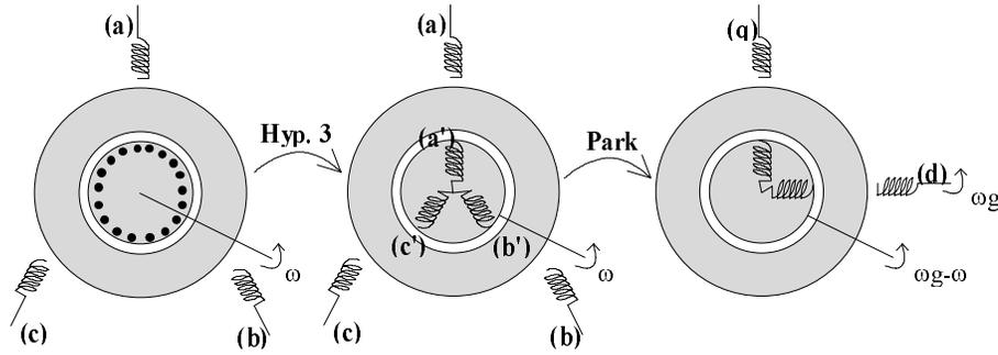
Fig. 1. Single cage induction machine modeling.
