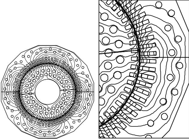
**Fig. 8.** Flux distribution at the maximum of short circuit torque.
