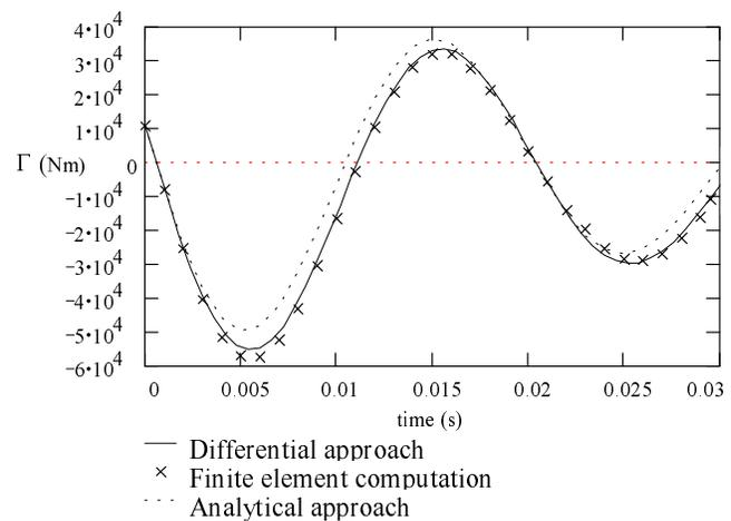
**Fig. 10.** Three phase short circuit torque.
