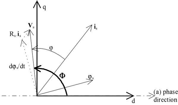
**Fig. 9.** Angular vector positions at the initial time of the short circuit.
