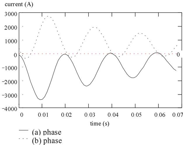
Fig. 5. Short circuit currents waveforms.
