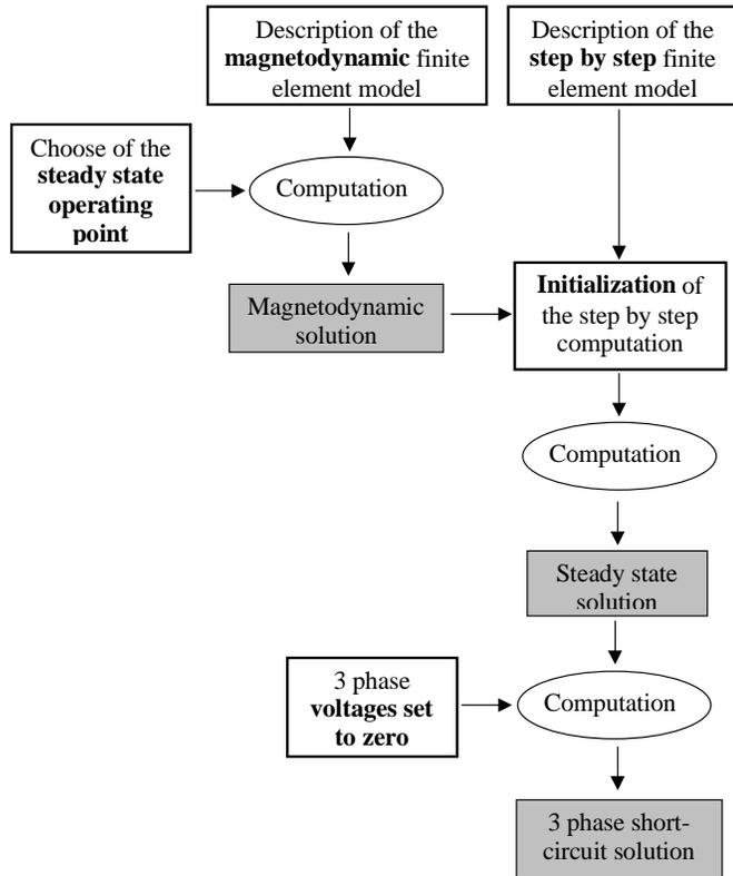
Fig. 4. Description of the finite element procedure.
