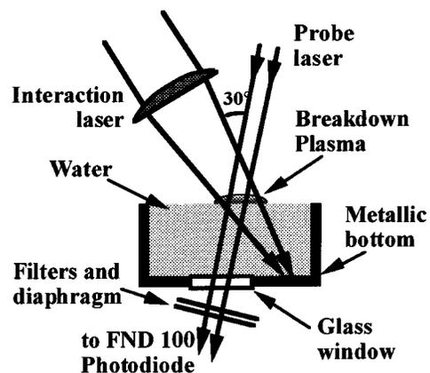
Fig. 1. Experimental set-up for transmission measurements.
