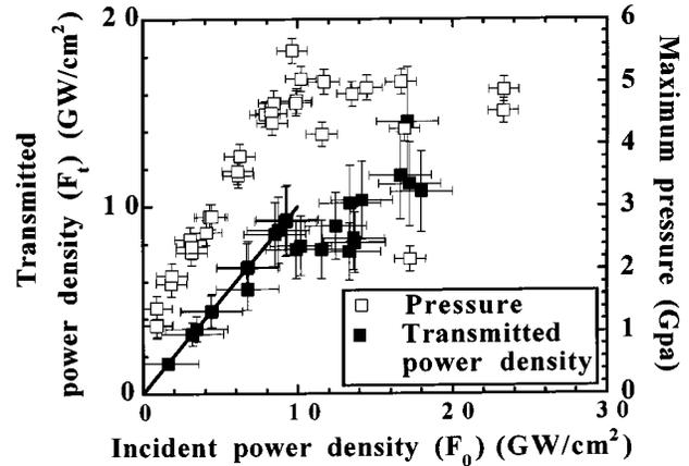
Fig. 4. Peak pressure measurements from reference [4], and transmitted power density  $F_t$  as a function of incident power density  $F_0$ .
