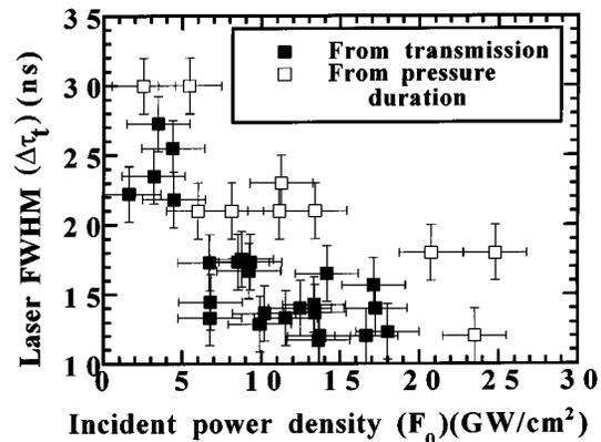
Fig. 5. Transmitted FWHM laser pulse ( $\Delta\tau_t$ ) as a function of incident power density from transmission experiments and determined from the pressure duration measurements (from Ref. [4]).
