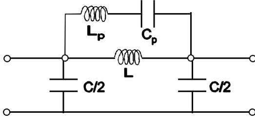
Fig. 8. Secondary mode line: one turn equivalent scheme.
