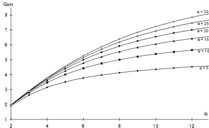
Fig. 11. Theoretical  $Gg^{(N)}$  versus  $N$  for some ratios  $a = Z_2/Z_0$ .
