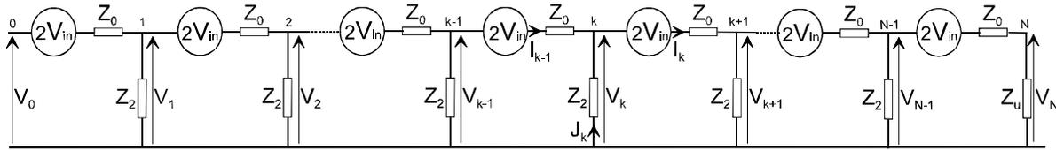
Fig. 9. Voltage gain calculation: T.L.T. equivalent scheme.
