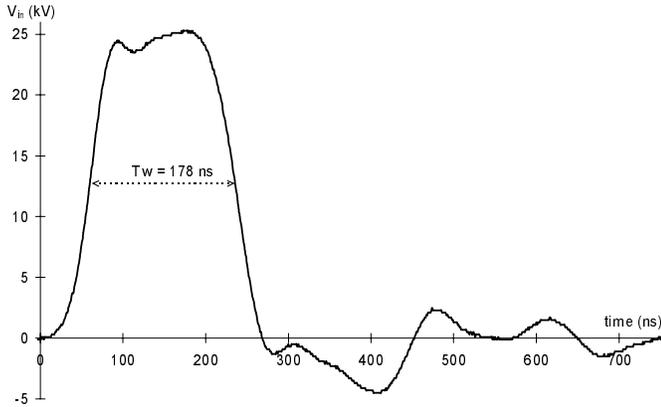
**Fig. 13.** Blumlein output pulse ( $d/w \approx 0.91$ ;  $L = 41$  nH;  $12.5 \Omega$ ).
