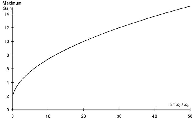
Fig. 10. Theoretical  $Gg^\infty$  versus  $Z_2/Z_0$  ratio.
