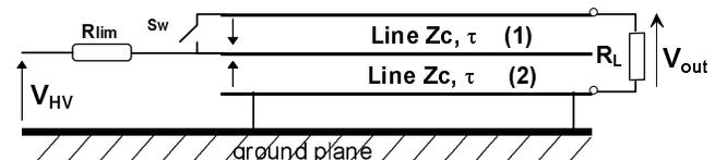
Fig. 1. Blumlein generator principle.
