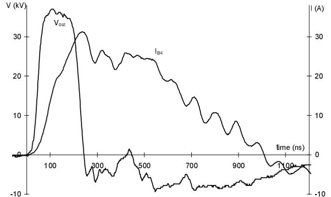
**Fig. 14.** Output pulse and fourth cable braid current shapes.
