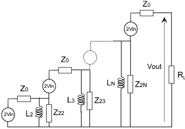
**Fig. 7.**  $N$  stage transmission line transformer equivalent scheme.
