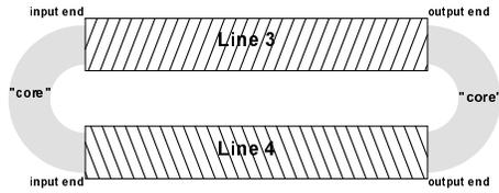
**Fig. 15.** Winding diagram of the TLT lines 3 and 4 (*idem* lines 1 and 2).
