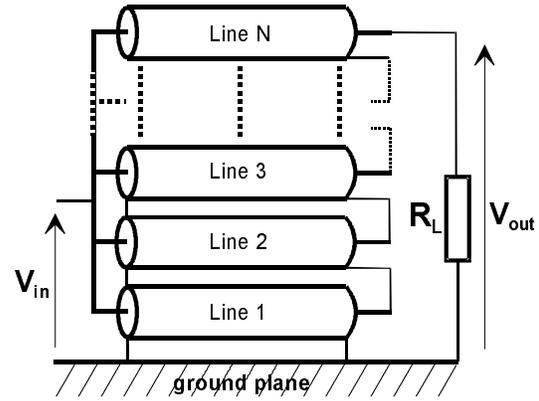
**Fig. 6.** Transmission line transformer principle.
