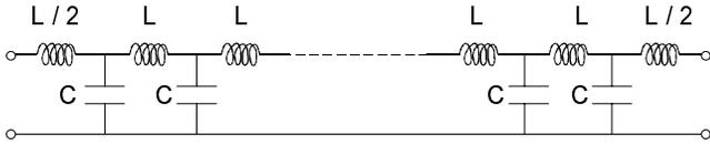
Fig. 2. Blumlein generator line principle.
