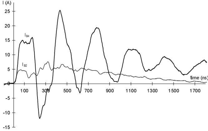
**Fig. 16.** Second and fourth cable braid current shapes.
