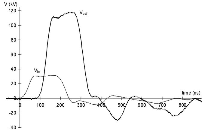
**Fig. 18.** Generator input and output pulses.
