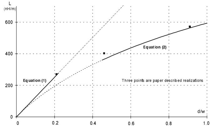
Fig. 3. Theoretical and measured inductance values versus  $d/w$  ratio.
