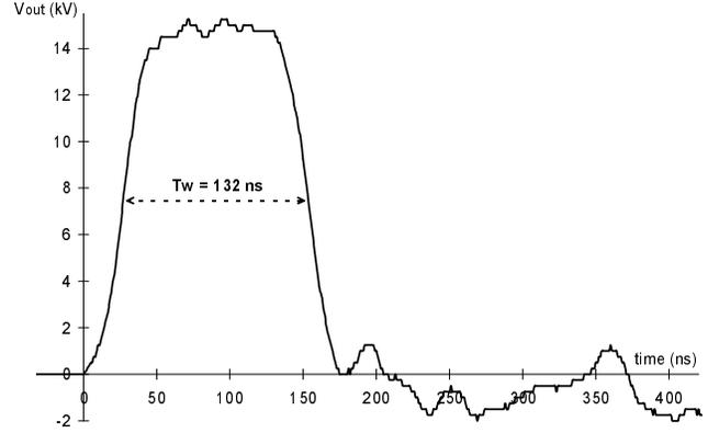
**Fig. 5.** Blumlein output voltage ( $d/w \approx 0.48$ ;  $L = 12$  nH;  $12.5 \Omega$ ).
