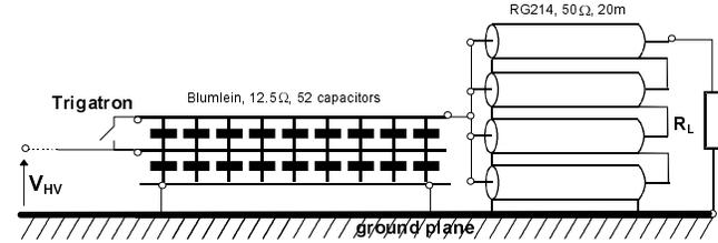
Fig. 12. Transmission line generator principle.
