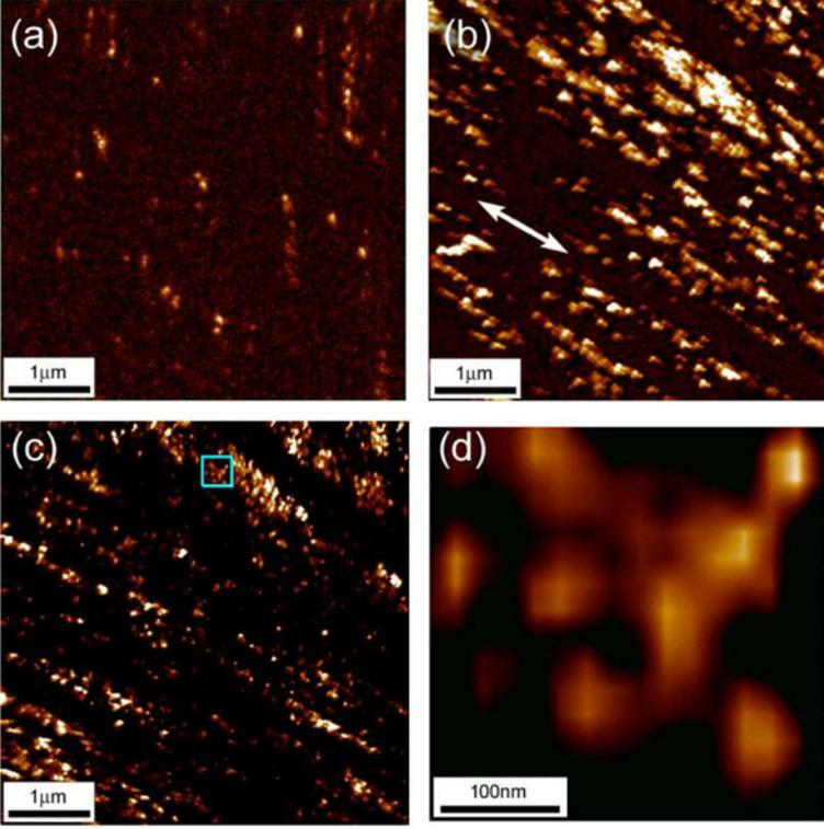
**Fig. 3.** (Color online) Typical SSRM images of the (0001) surface of (a) undeformed and (b)–(d) deformed samples. Here, we used a conductive diamond tip with the tip bias of +9 V. The images of (b) and (c) are from different positions on the same sample, and an area indicated by a square in (c) is enlarged and shown in (d). The arrow in (b) indicates the slip direction.
