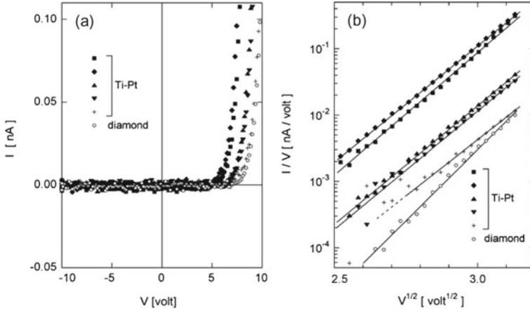
**Fig. 4.** (a) Local ( $I$ - $V$ ) spectra measured at the positions of conductive spots in SSRM images using a conductive diamond-coated tip and a Ti-Pt-coated tip, (b) the data in (a) are re-plotted as  $\log(I/V) - V^{\frac{1}{2}}$ .
